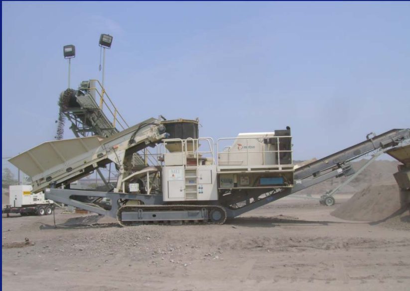
4-inch nominal slag crusher at Sparrows Point Steel Mill
